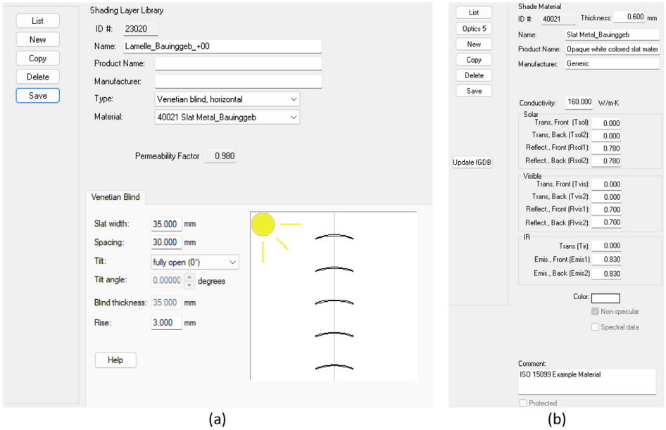
Fig. 5. Definition of the venetian blind system in the reference office space in the WINDOW software: (a) Specification of the geometry, (b) specification of base material.
